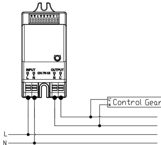
\*The sensor is designed for connect one load only. Connect more than one loads may damage the sensor.
